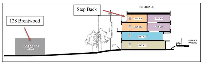
Figure 5 – Cross-Section Showing Relationship of the Proposed Building to Brentwood Homes (Note: Step back of the top level)
