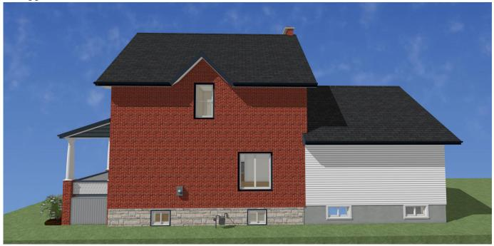
Addition to be framed with 2x6 exterior studs @ 16"o/c, while interior walls will be framed with 2x4 studs @ 16"o/c. Horizontal Gentek siding in "Snow White 001" to best match what was installed on the previous addition. The siding is to be Double 4" Clapboard.
