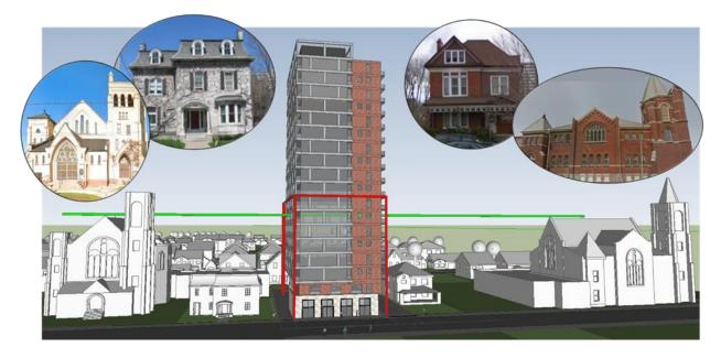
Figure 8: The applicant-proposed build amidst the existing streetscape as depicted in the City of Kitchener 3-D conceptual model. The red lines depict the maximum building envelope under the City-proposed Secondary Plan. The green line shows the height of the peak of the church roofs relative to the applicant-proposed build.
