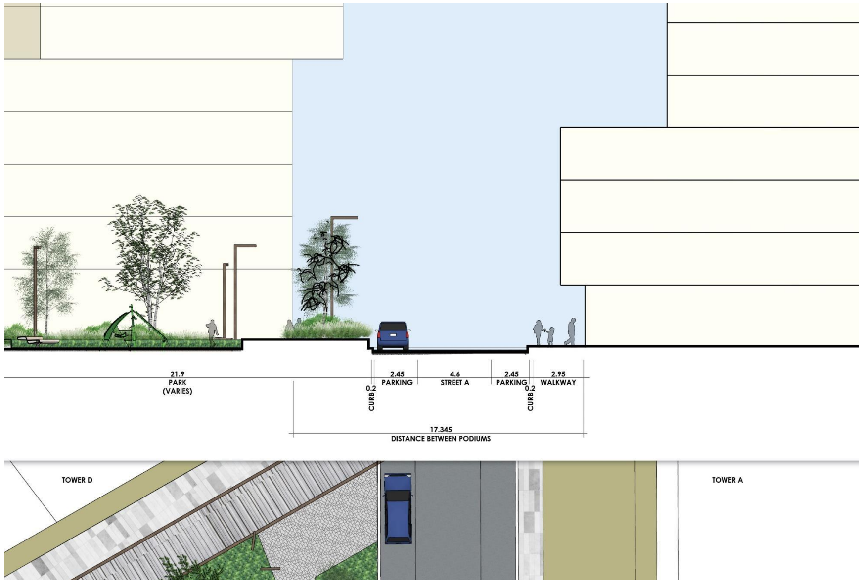
Figure 38: Cross Section of Street A - One-way laneway (Land Art, February 2023)
