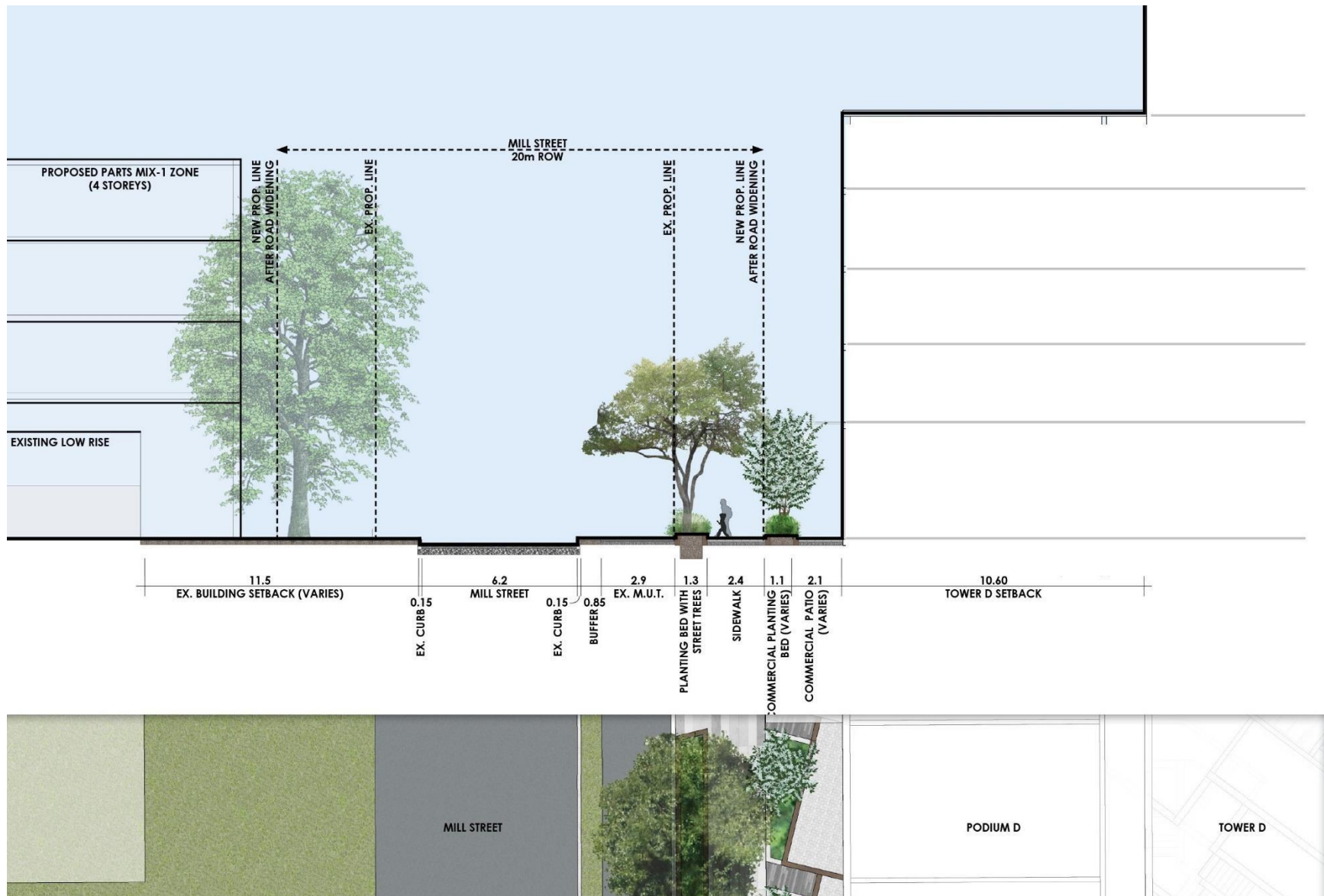
Figure 36: Mill Street Cross Section - 20m Right-of-Way (Land Art, February 2023)
