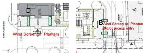
Given the broad extent of Building B, the main (west) entry can be impacted by downwash winds stream-lined along Lancaster. This entry should be flanked by wind-mitigation devices (Figure 7) or adequately set-back from the building face.
