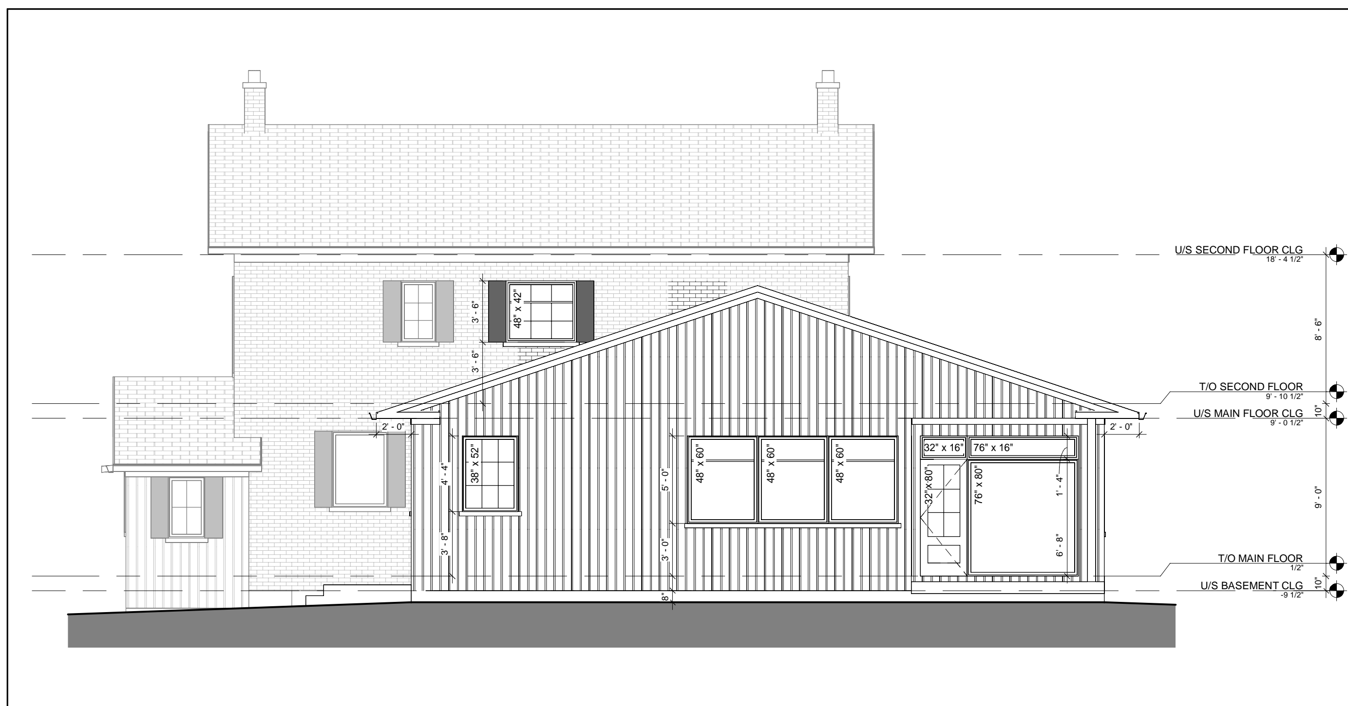
2 SOUTH ELEVATION - NEW CONSTRUCTION 3/16" = 1'-0"
