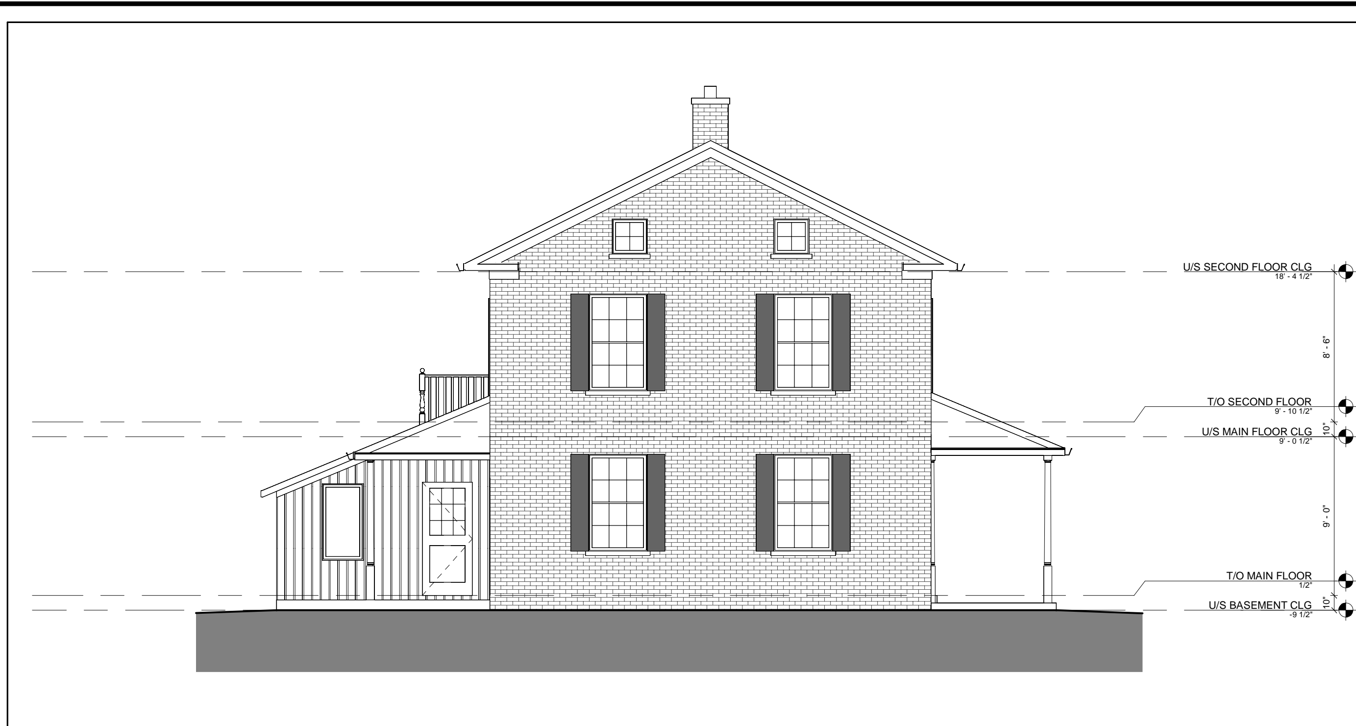
1 EAST ELEVATION - EXISTING AND DEMOLITION 3/16" = 1'-0"
