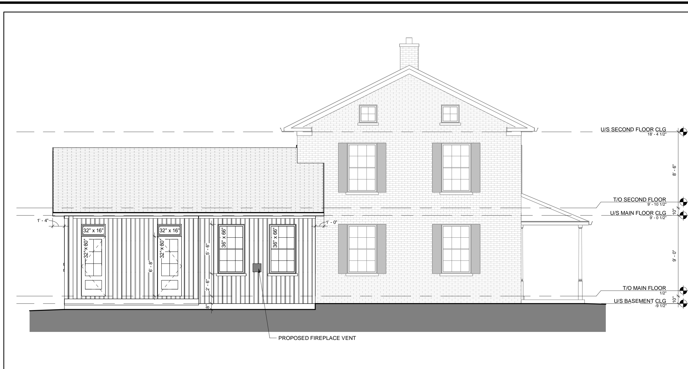
1 EAST ELEVATION - NEW CONSTRUCTION 3/16" = 1'-0"
