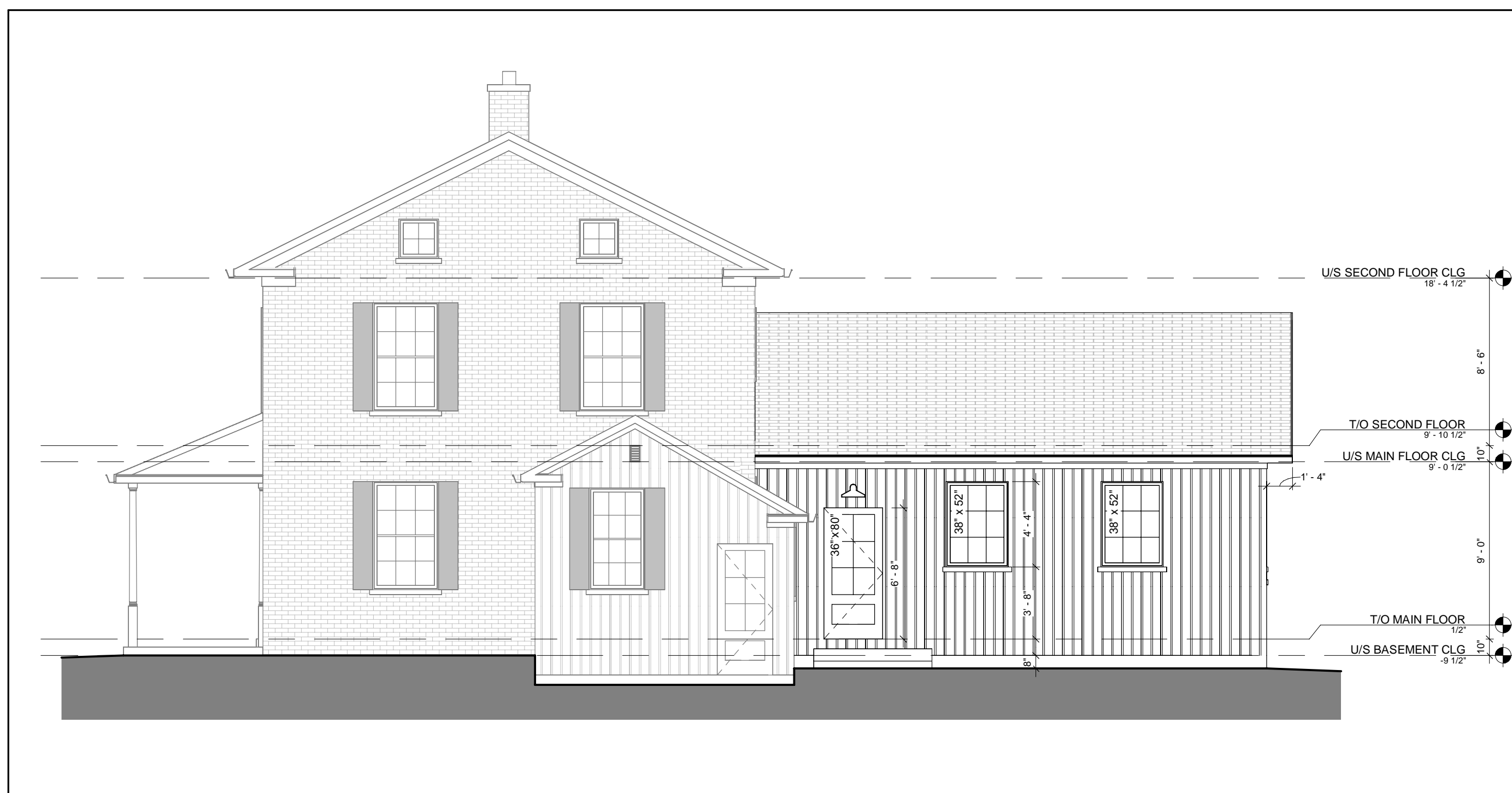
2 WEST ELEVATION - NEW CONSTRUCTION 3/16" = 1'-0"
