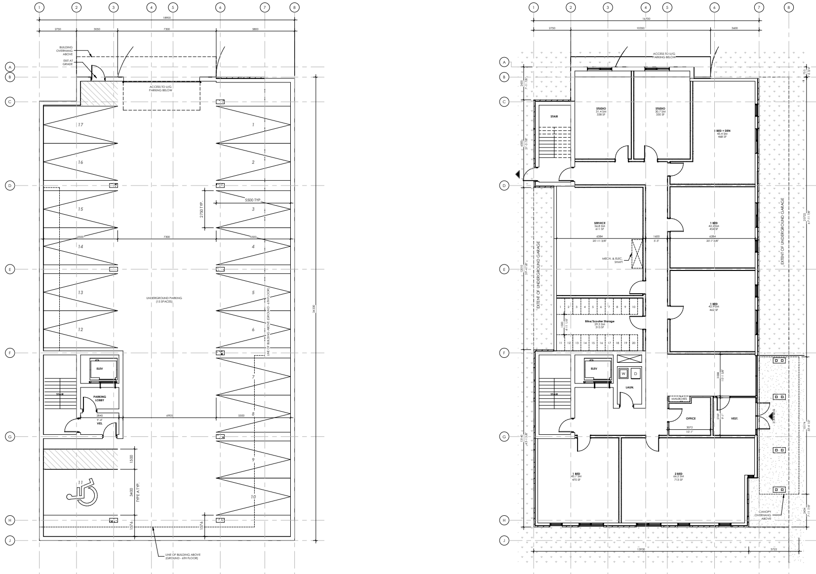
Figure 34. Underground Parking Plan (left) and Ground Floor Plan (right) of the proposed development. (Source: EDGE Architects, April 2023)
