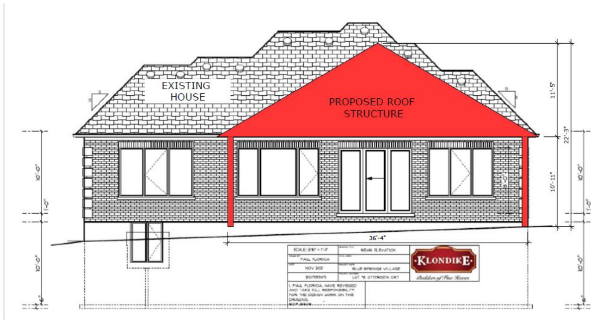
Figure 4: Elevation view of the covered structure
