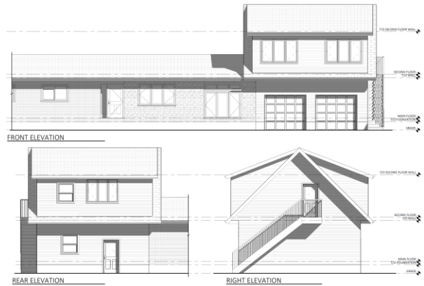
Elevation drawings showing the proposed addition to the existing single detached dwelling
