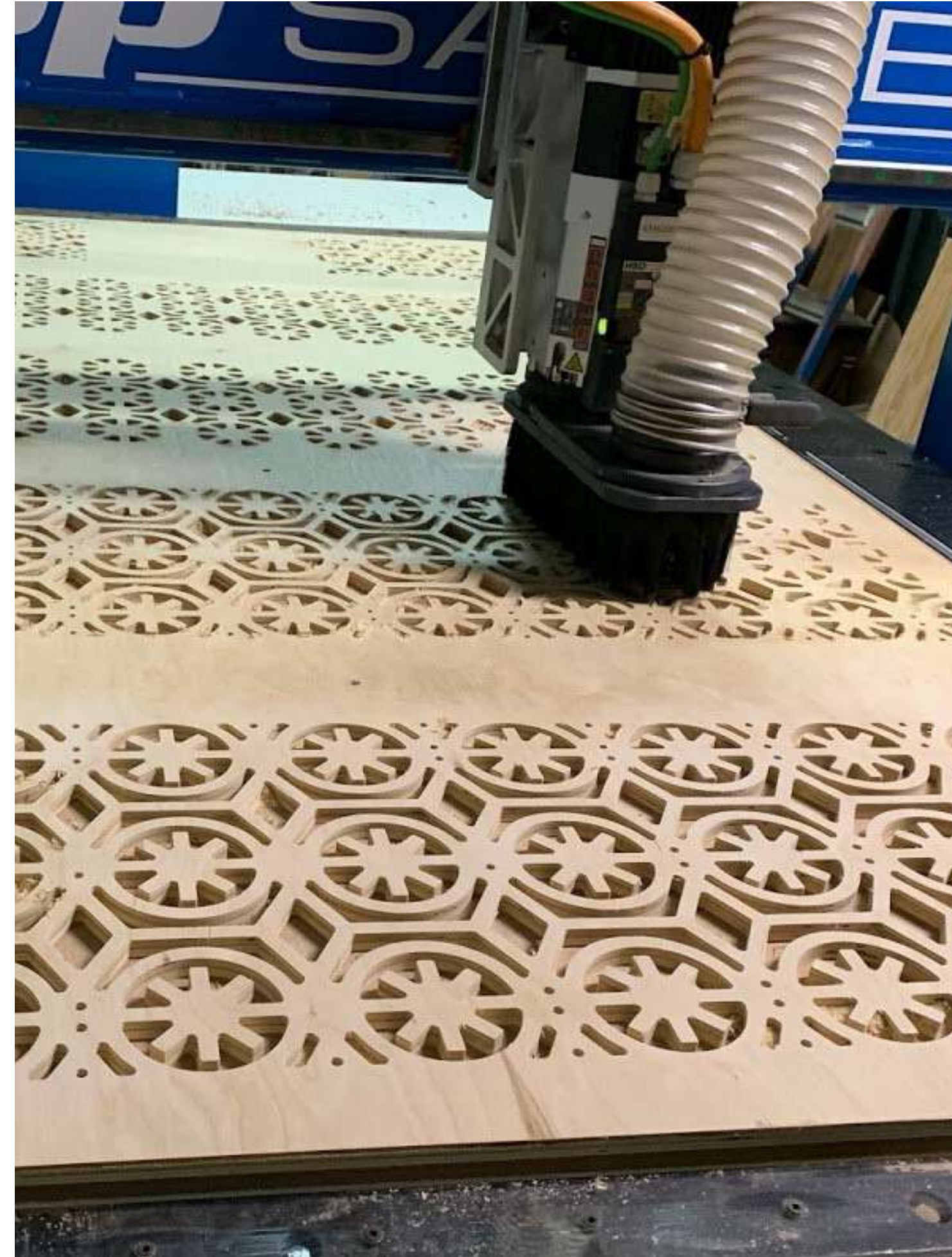
PLYWOOD PANELS ARE CUT WITH A CNC MACHINE TO CREATE THE IMAGERY
