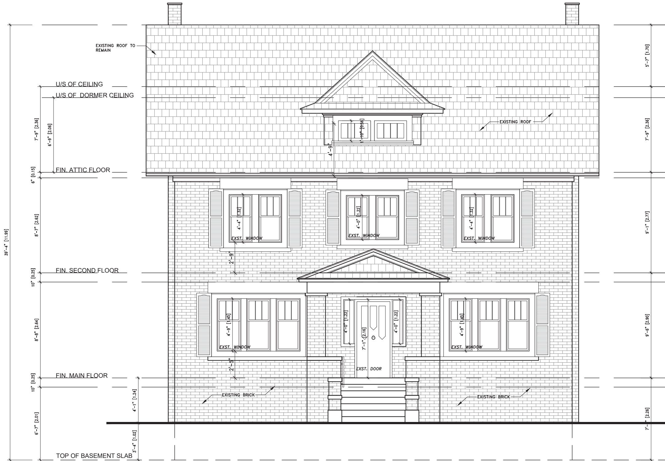
PROPOSED FRONT ELEVATION SCALE: 3/16"=1'-0"
