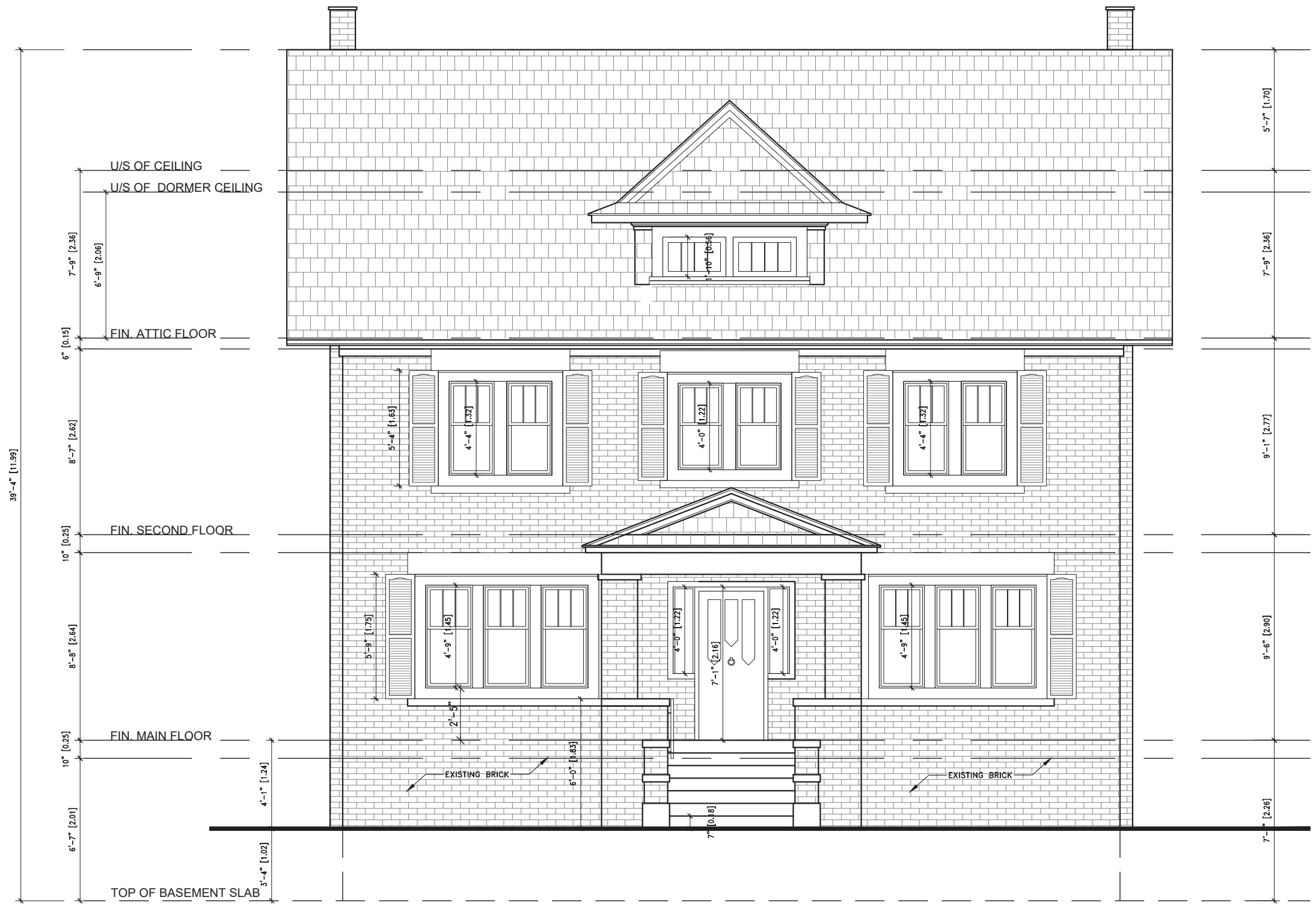
FRONT ELEVATION SCALE: 3/16"=1'-0"
