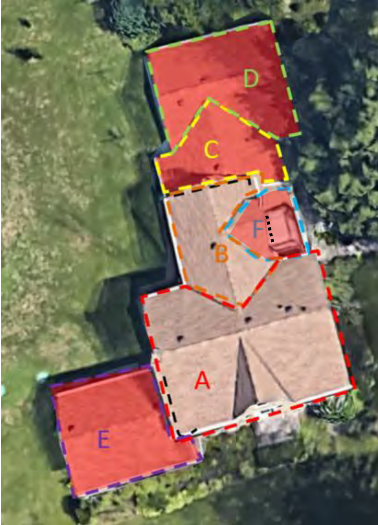
Figure 3: Aerial image of existing dwelling, noting the contemporary additions to the dwelling which are proposed for removal (shaded in red). Elevations which may require alteration following the removal of contemporary additions noted with dashed black lines. (Source: MHBC, 2023)
