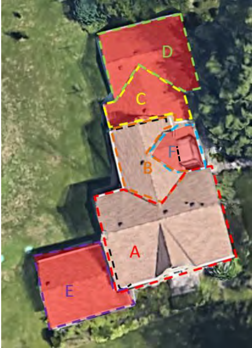
Figure 1: Aerial image of existing dwelling, noting the contemporary additions to the dwelling which are proposed for removal (shaded in red). Elevations which may require alteration following the removal of contemporary additions noted with dashed black line. (Source: MHBC, 2023)
