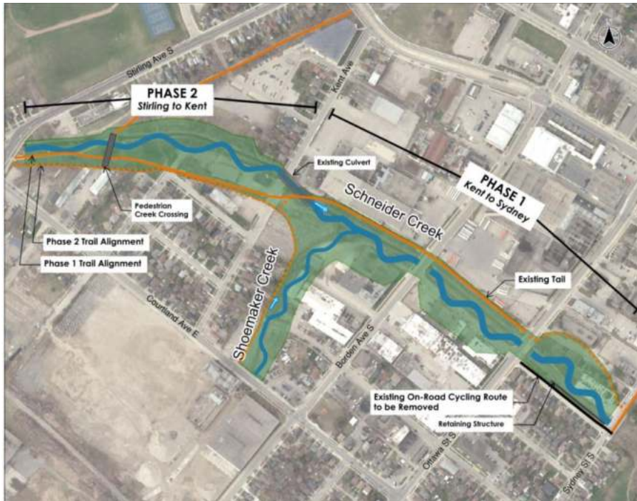
Figure 3.3: Multi-Use Trail along a Combination of the North and South side of Schneider Creek and West side of Shoemaker Creek
