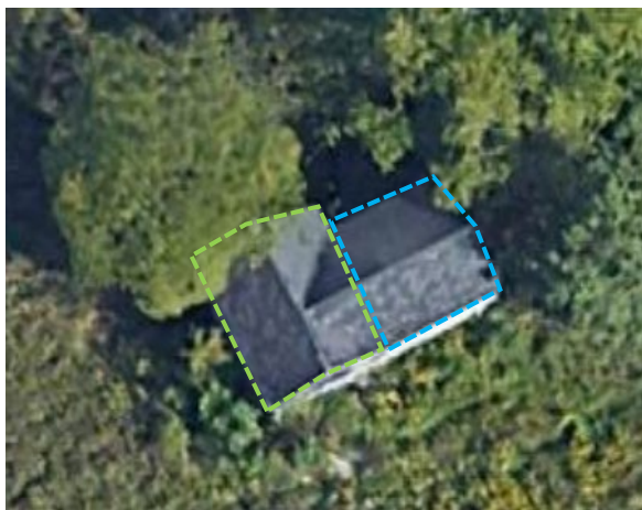
Figure 17: Aerial view of the house. Green dashed line indicates original log house, blue dashed line indicates later additions (Google, 2023)
