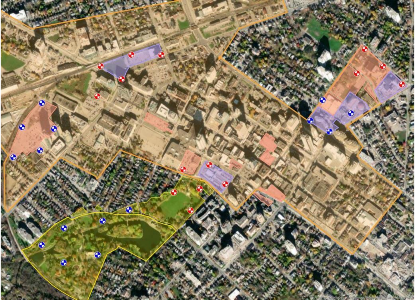
Figure 11: Salas O’Brien Open Loop Well Locations
