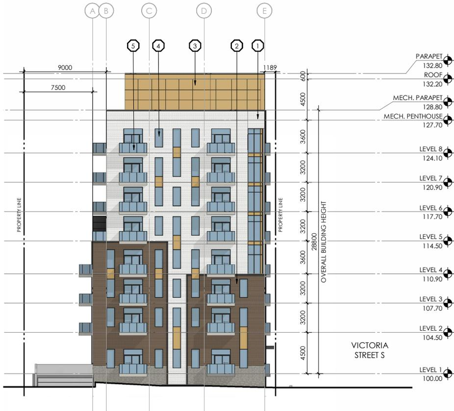
Fig.19: East elevation
