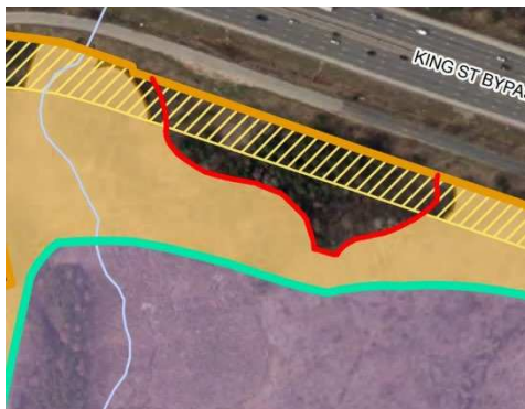
Figure 6d: NRSI constraints mapping with Jefferson Salamander Regulated Habitat (teal line), proposed area of retained Jefferson Salamander Habitat (purple), overall constraints of NHS (wetland buffer) in red. Tan area is a designated 'enhancement area' between JESA habitat and outer NHS buffer. Cross hatched area is the zone of impact from the Hidden Valley Road upgrades in this area
