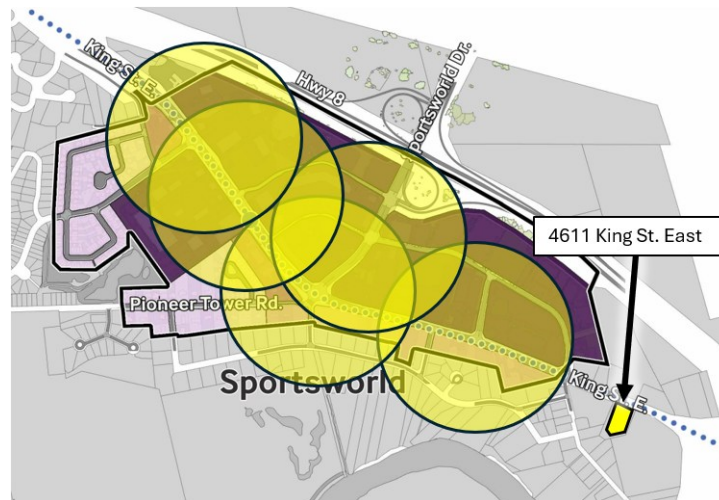
Figure 4 – All Sportsworld area pedestrian crossings visualized with 300m radius with PMTSA outlined. Complete Streets Kitchener defines 'greater than 300m' distance to a crossing as 'no level of service'.
