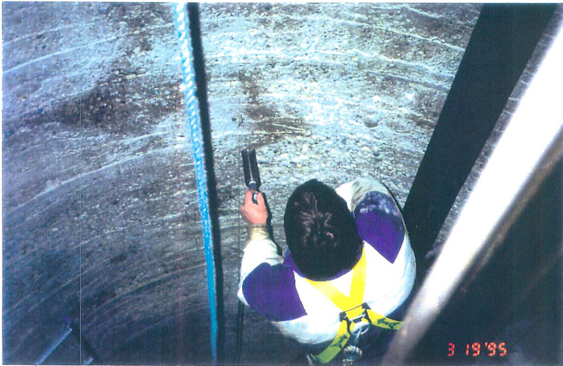
Impact-echo testing the inside walls
