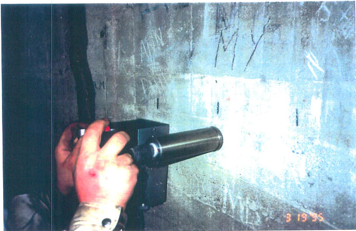
Evaluating the P-wave speed using two impact-echo heads
