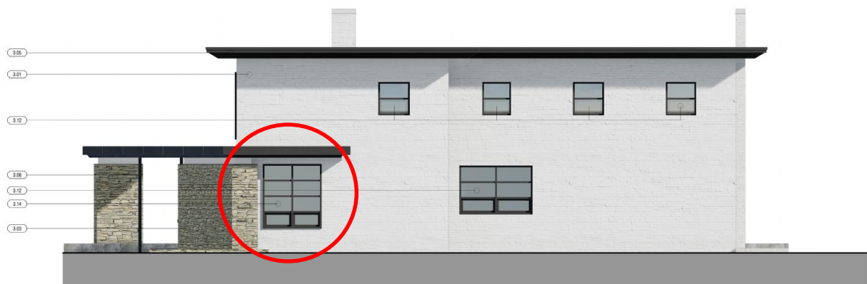
Figure 4: Architectural Drawing of South Façade with Proposed Alterations. Window to be Replaced Circled.
