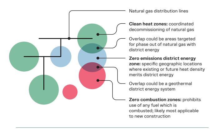
Figure 10. Illustration of land-use zones for decarbonization of heat.
