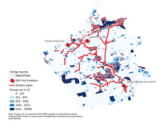
Figure A4.3. Energy density, sanitary pipes, and potential district energy hubs.
