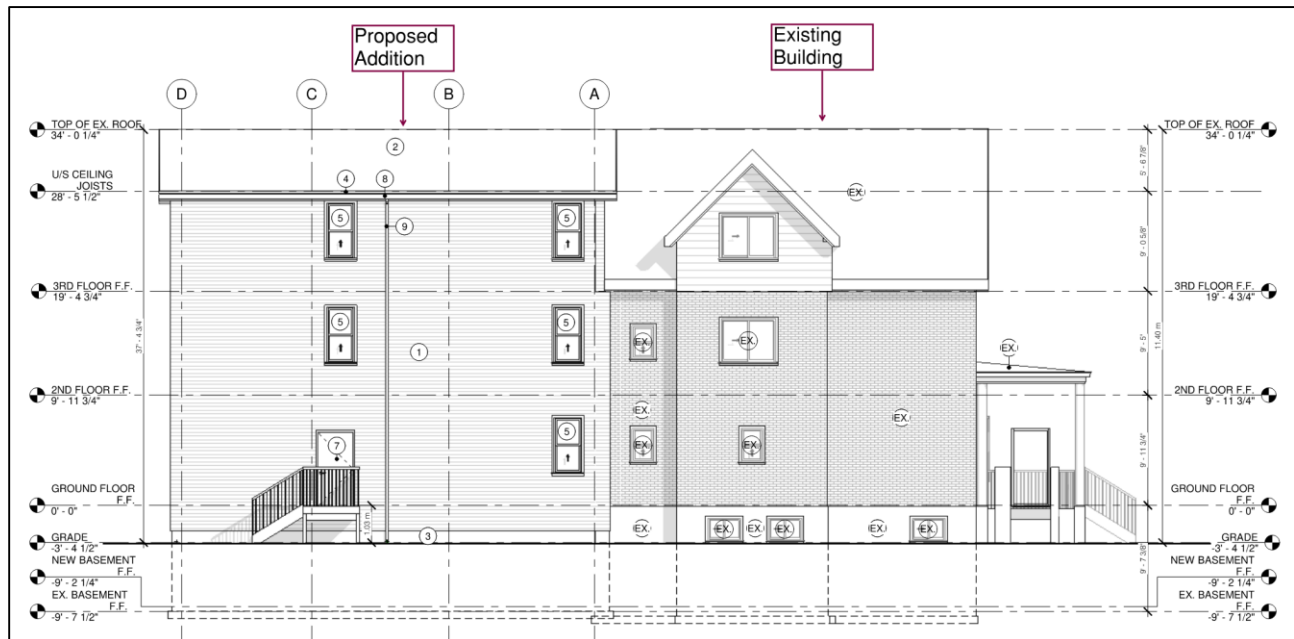
Figure 4 – Proposed east elevation drawing, showing the existing building (right) and proposed rear yard addition (left).
