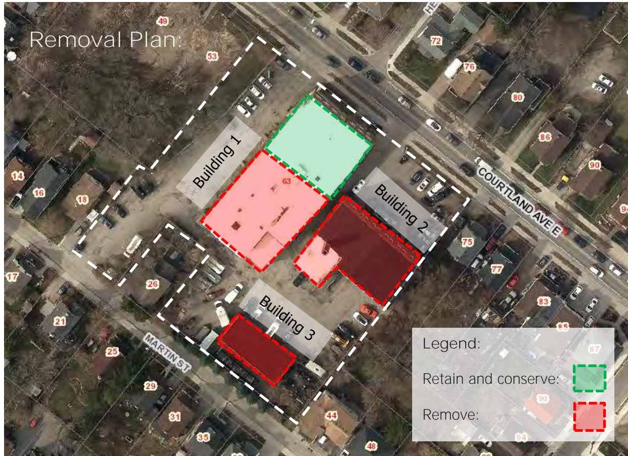
Figure 47: Aerial photo noting the location of the subject property at 63 Courtland Avenue East, outlined in white. Location of building fabric proposed for demolition noted in red (demolish) and retention noted in green. (Source Kitchener Interactive map, accessed 2024)
