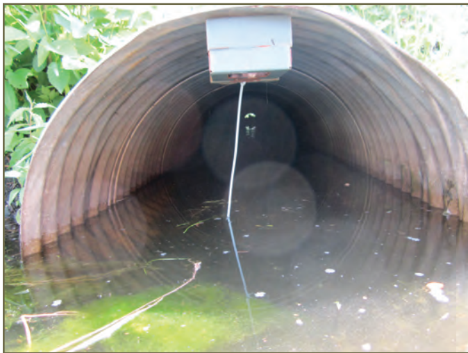
Photo 66. Camera securely fastened to top of culvert; note difficult to capture animals when water in culvert or tunnel. © K. Gunson
