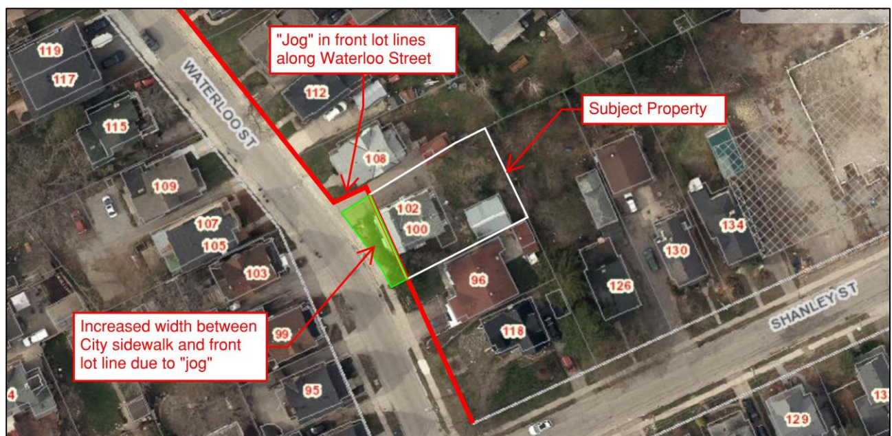
Figure 2: Plan showing the “jog” in the front lot lines along Waterloo Street in the vicinity of the subject property, which creates increased width between the City sidewalk and the front lot line.
